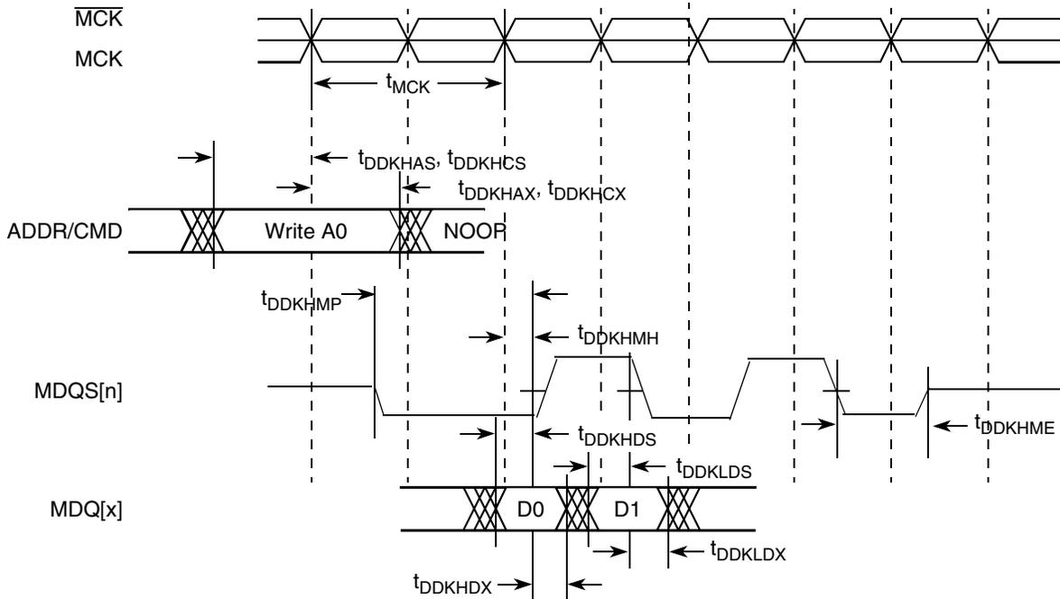
**Figure 10. DDR2 and DDR3 Output Timing Diagram**
