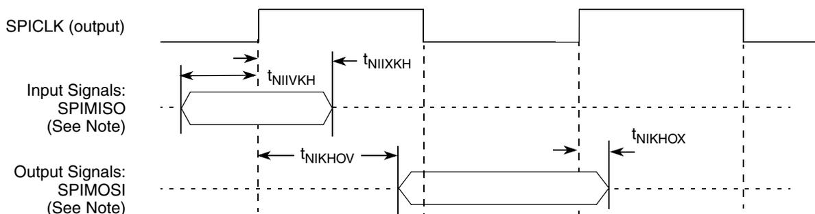
**Note:** The clock edge is selectable on SPI.
