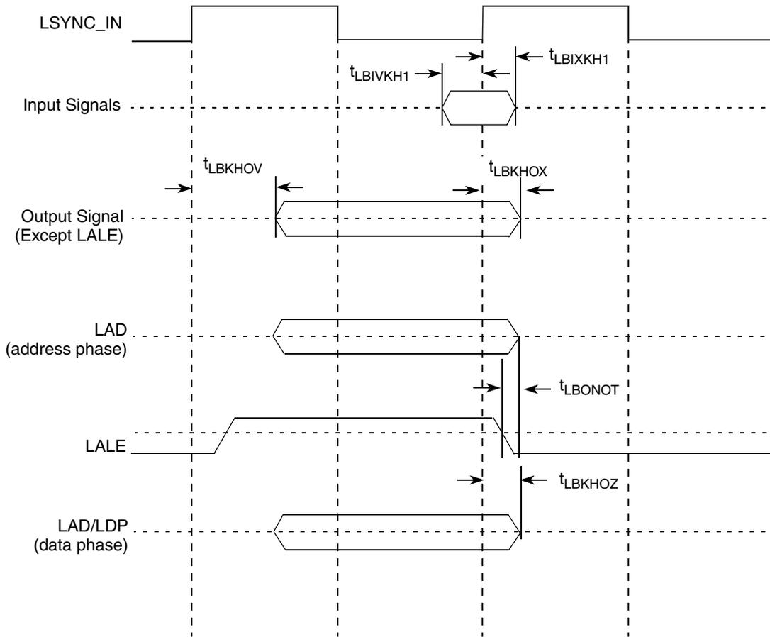
**Figure 57. Local Bus AC Timing Diagram (PLL Enabled)**
