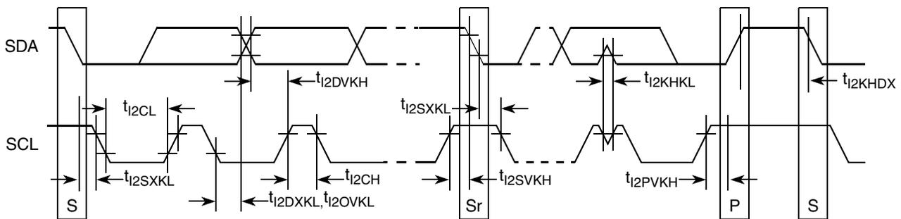
**Figure 50. I<sup>2</sup>C Bus AC Timing Diagram**
