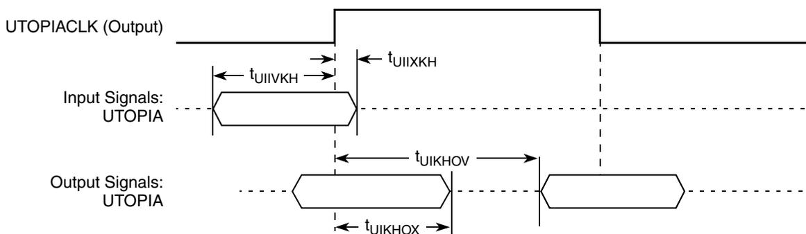
Figure 72. UTOPIA/POS AC Timing (Internal Clock) Diagram
