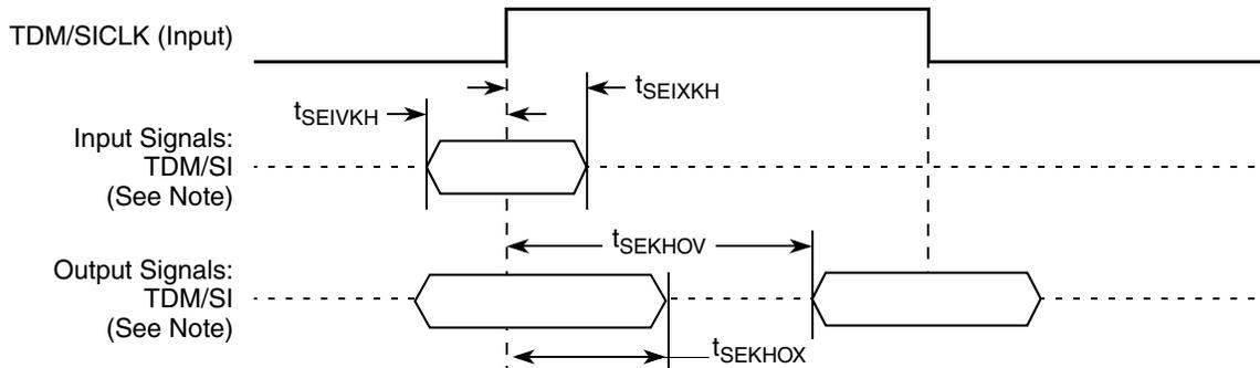
**Note:** The clock edge is selectable on TDM/SI.
