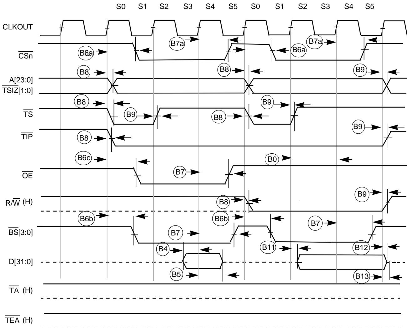
Figure 11. Read/Write (Internally Terminated) SRAM Bus Timing
