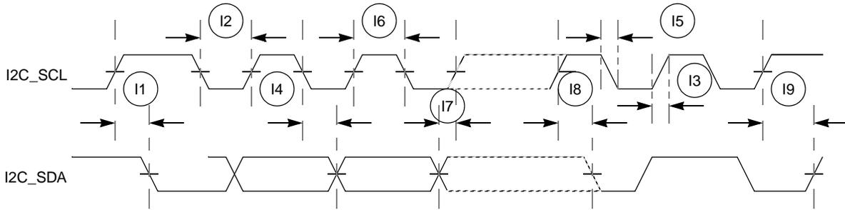
Figure 18. I<sup>2</sup>C Input/Output Timings
