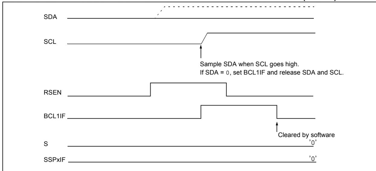
**FIGURE 32-37: BUS COLLISION DURING REPEATED START CONDITION (CASE 2)**
