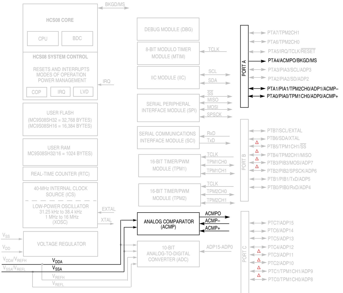
Figure 8-1. MC9S08SH32 Series Block Diagram Highlighting ACMP Block and Pins
