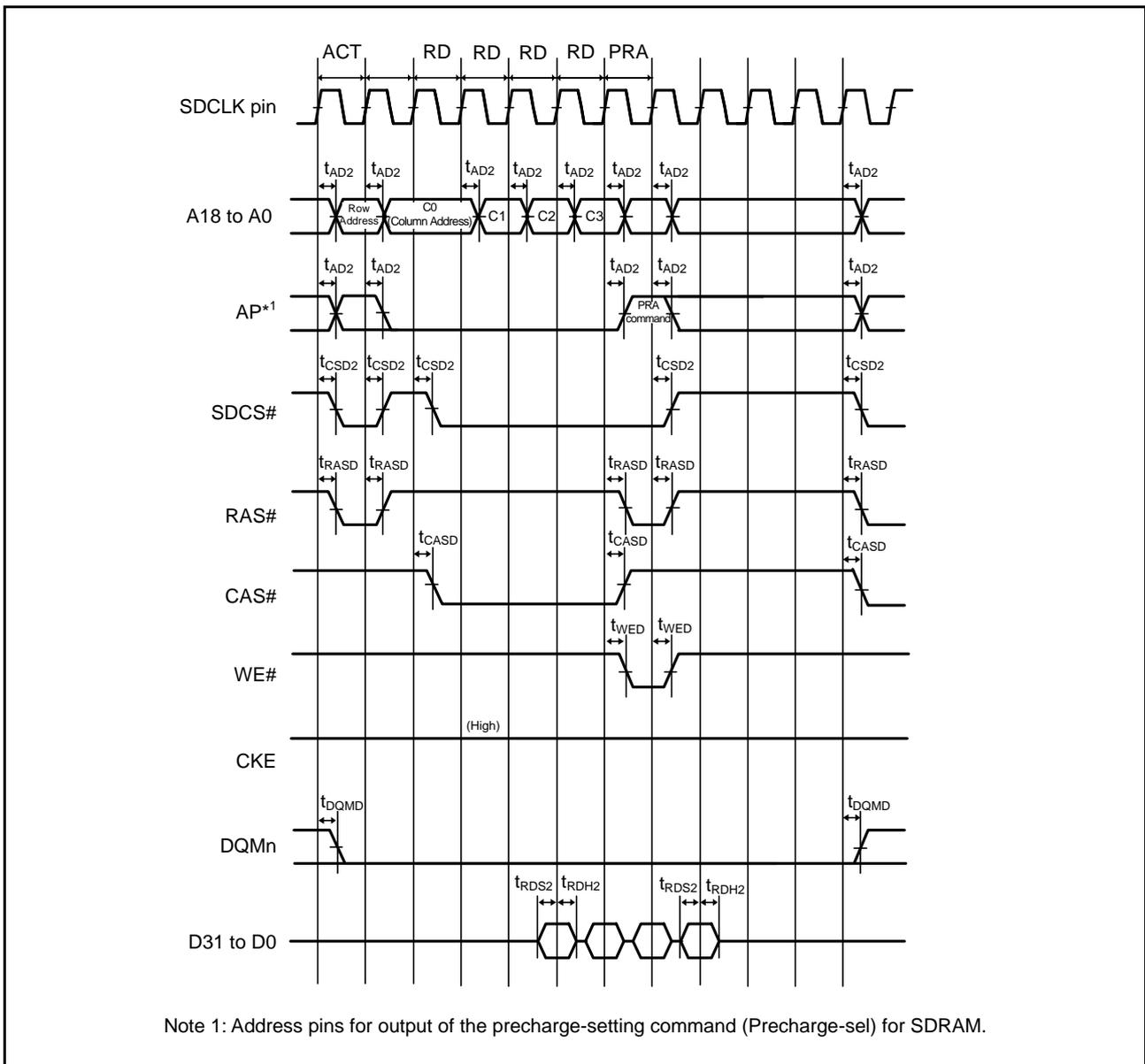
Figure 5.26 SDRAM Space Multiple Read Bus Timing
