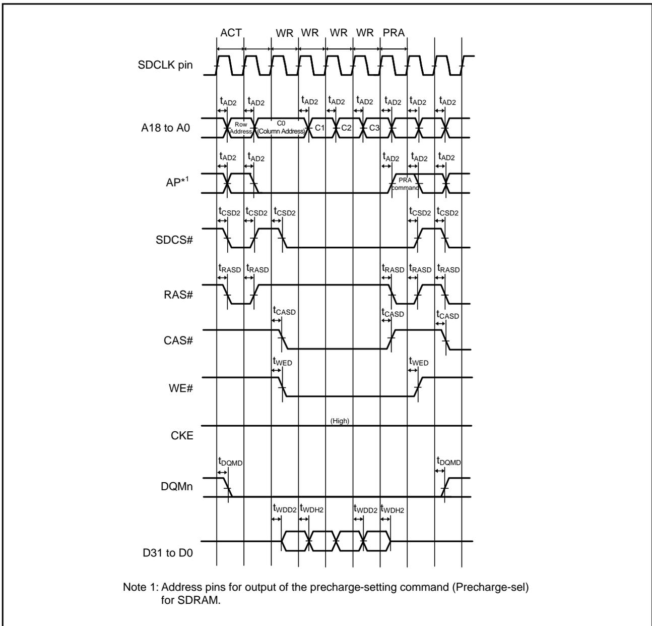
Figure 5.27 SDRAM Space Multiple Write Bus Timing
