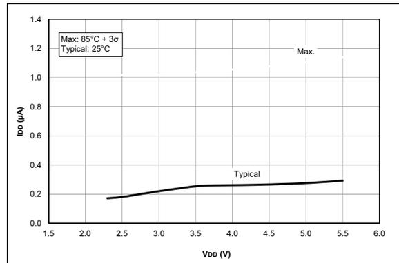
**FIGURE 35-48:**  $I_{DD}$ , ADC Non-Converting, PIC16F1717/8/9 Only.
