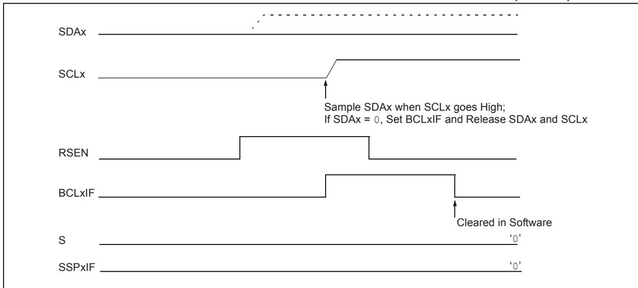
**FIGURE 20-32: BUS COLLISION DURING REPEATED START CONDITION (CASE 2)**
