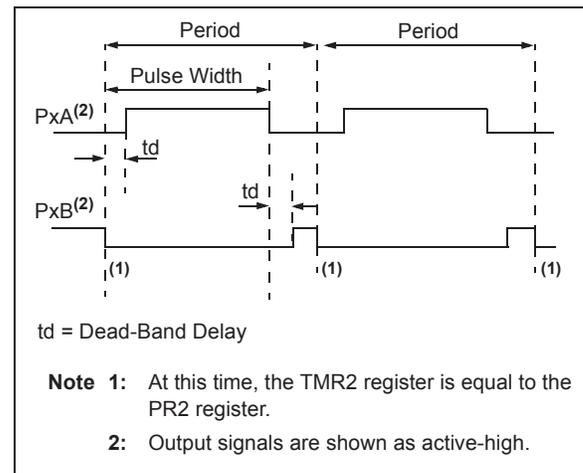
**FIGURE 19-15: EXAMPLE OF HALF-BRIDGE APPLICATIONS**
