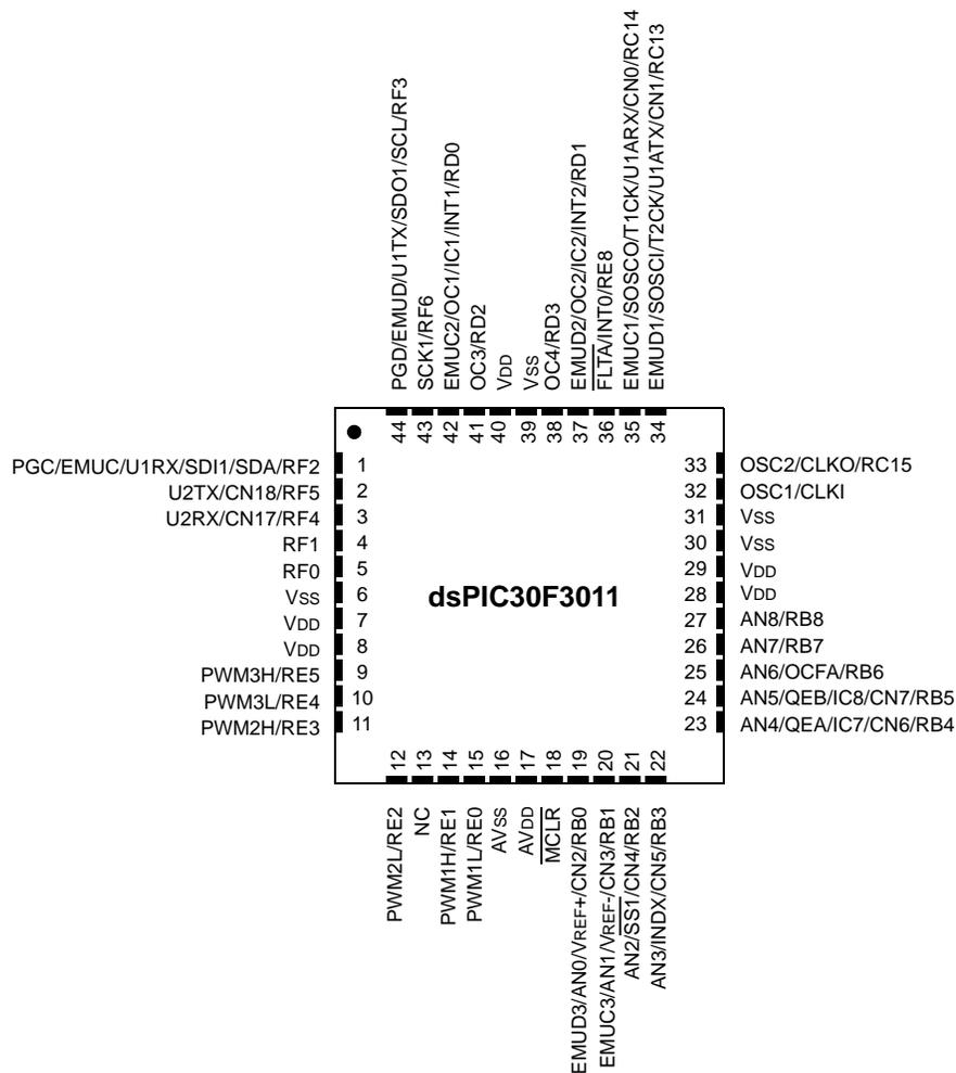
**Note 1:** The metal plane at the bottom of the device is not connected to any pins and is recommended to be connected to VSS externally.
