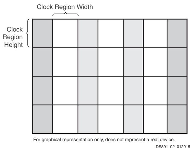
Figure 2: Column-Based Device Divided into Clock Regions
