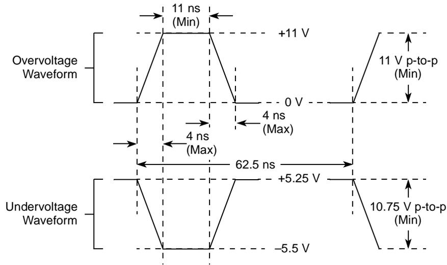
Figure 5. Maximum AC Waveforms for 5-V Signaling
