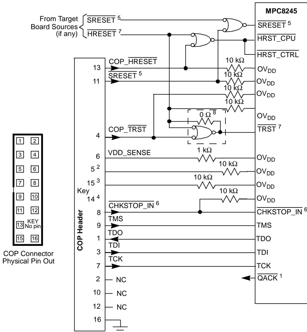
Figure 26. COP Connector Diagram
