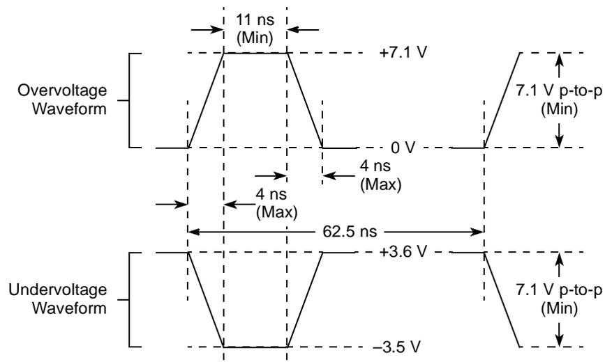
Figure 4. Maximum AC Waveforms for 3.3-V Signaling
