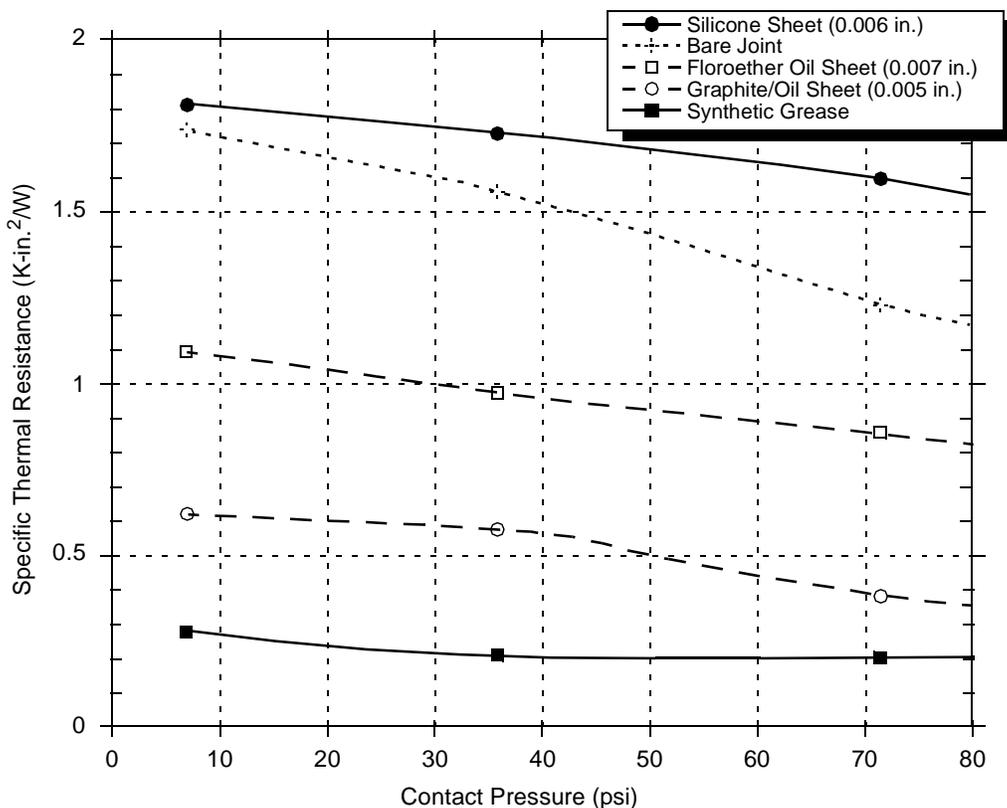
**Figure 30. Thermal Performance of Select Thermal Interface Material**
