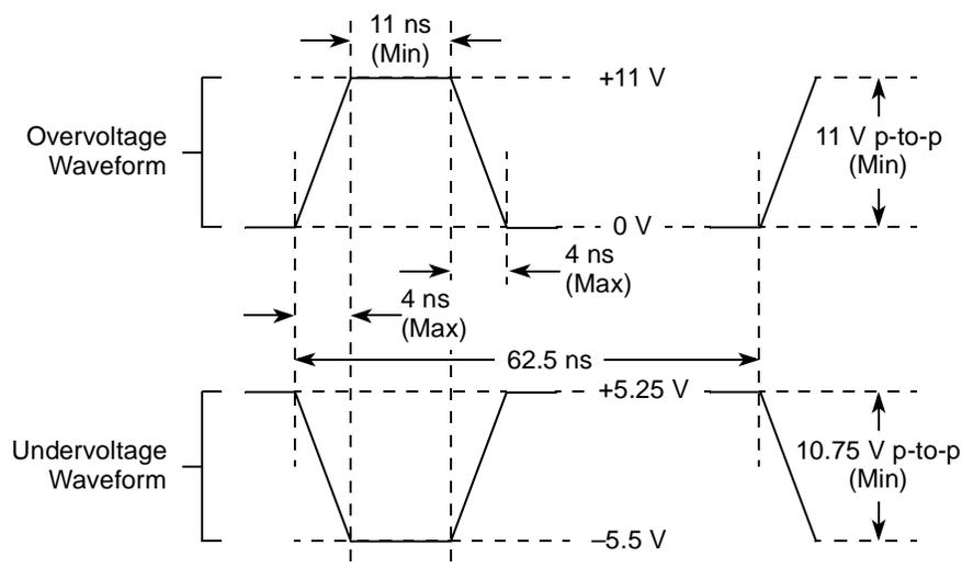
Figure 5. Maximum AC Waveforms for 5-V Signaling
