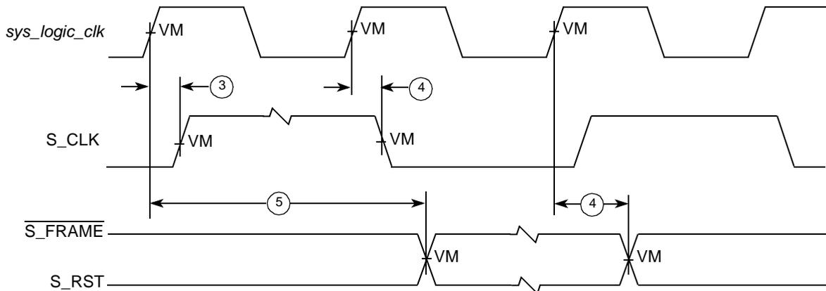
Figure 18. PIC Serial Interrupt Mode Output Timing Diagram
