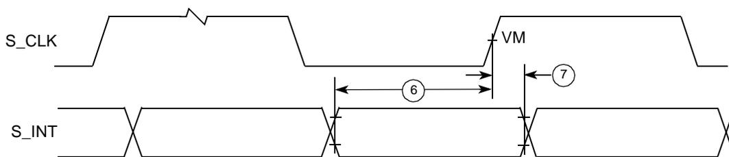
Figure 19. PIC Serial Interrupt Mode Input Timing Diagram
