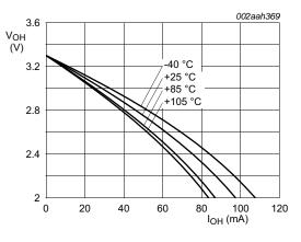
Conditions:  $V_{DD(REG)(3V3)} = V_{DD(IO)} = 3.3$  V; ultra high-drive; EHD = 0x3.
