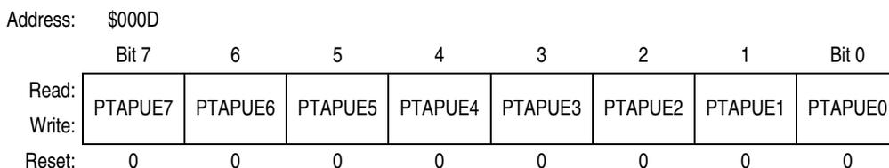
**Figure 13-5. Port A Input Pullup Enable Register (PTAPUE)**
