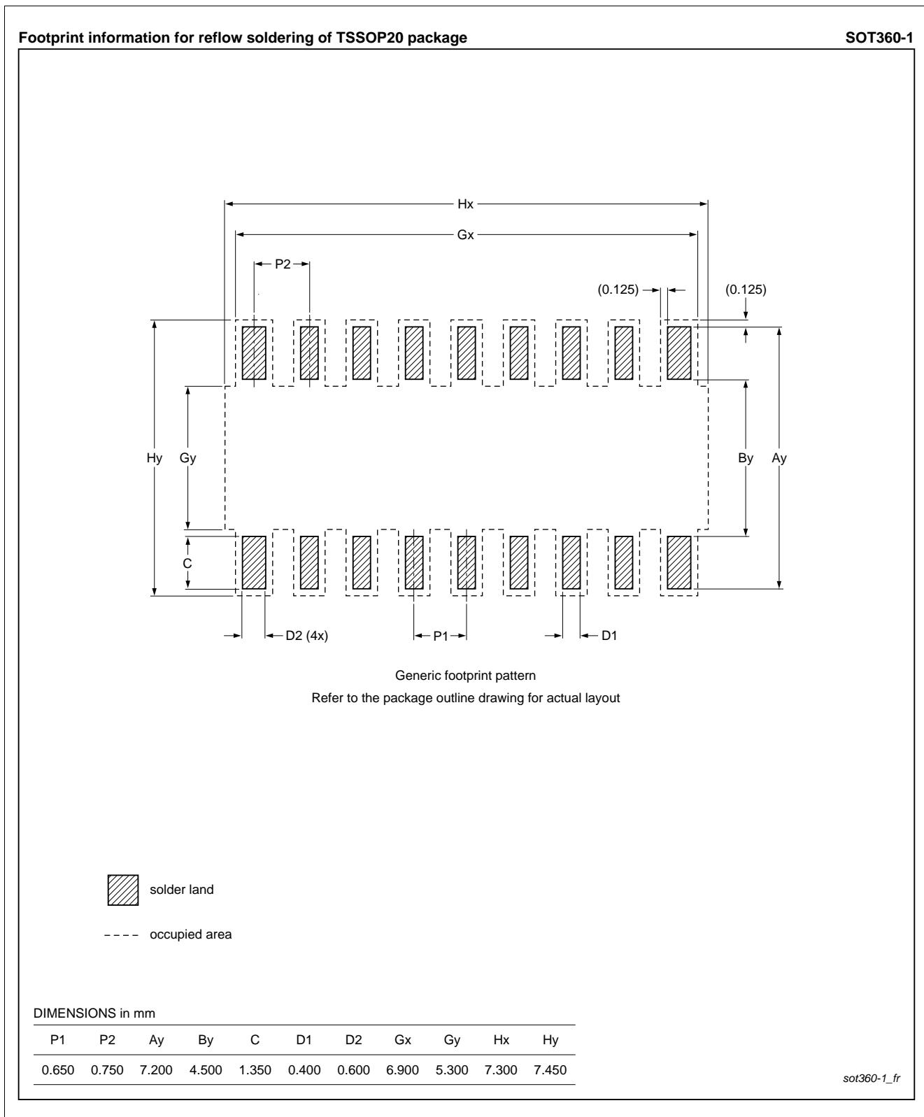
**Fig 64. Reflow soldering of the TSSOP20 package**
