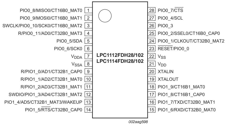
Fig 12. LPC1100L pin configuration TSSOP28 package
