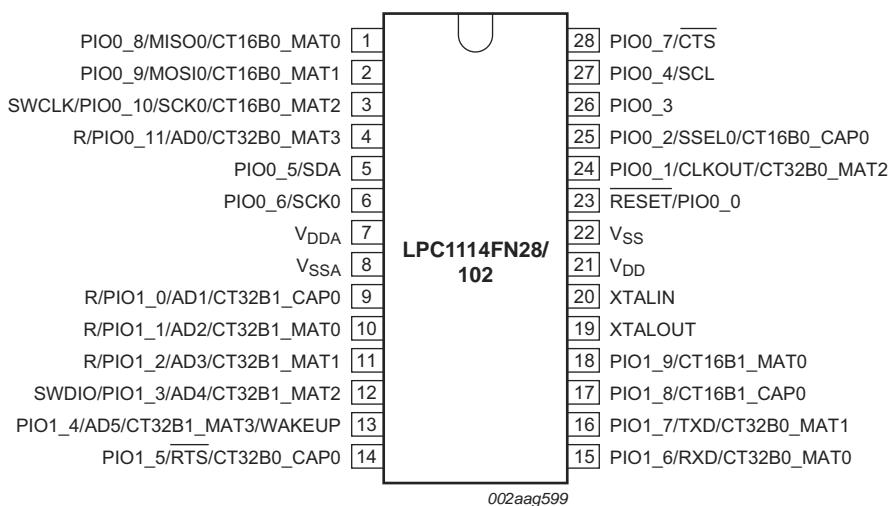
Fig 13. LPC1100L series pin configuration DIP28 package
