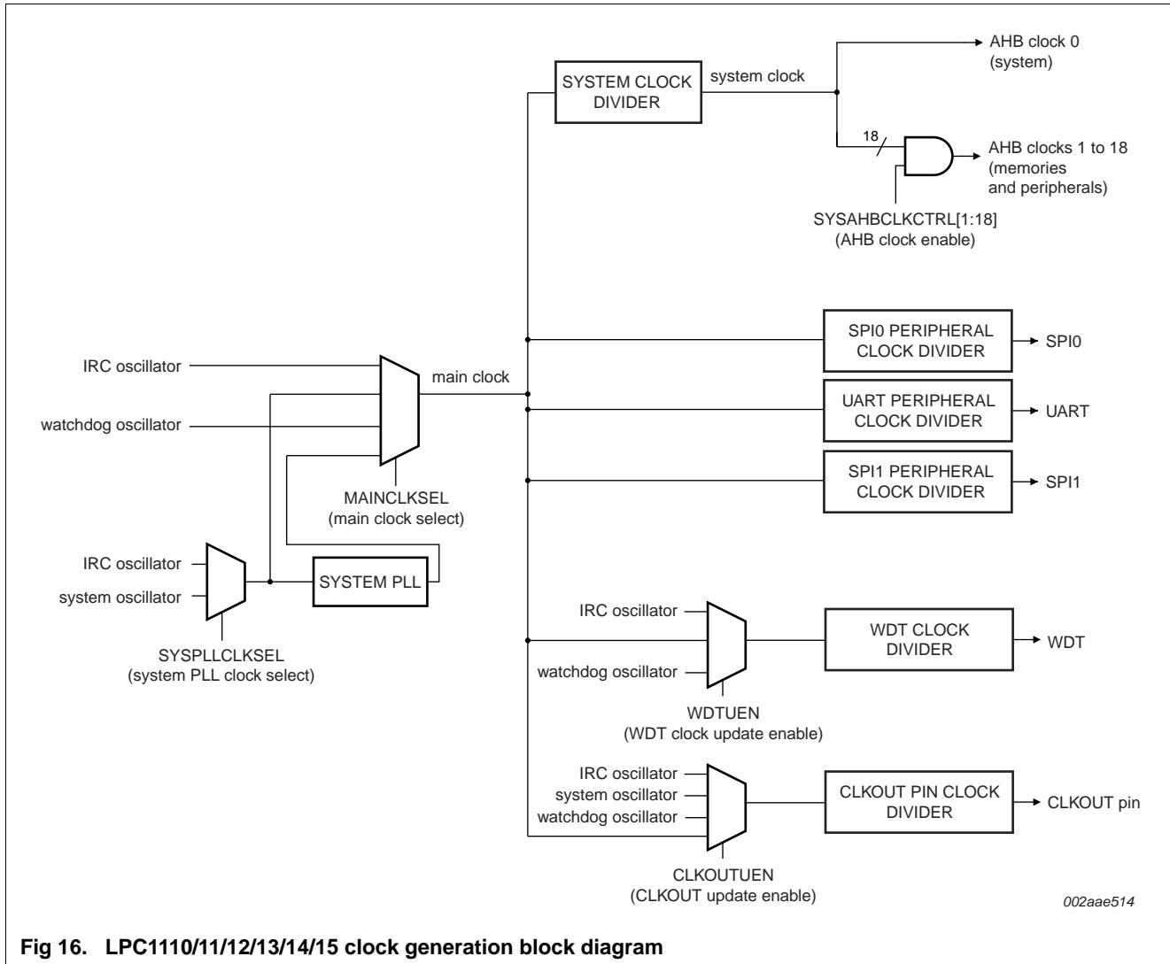
**Fig 16. LPC1110/11/12/13/14/15 clock generation block diagram**
