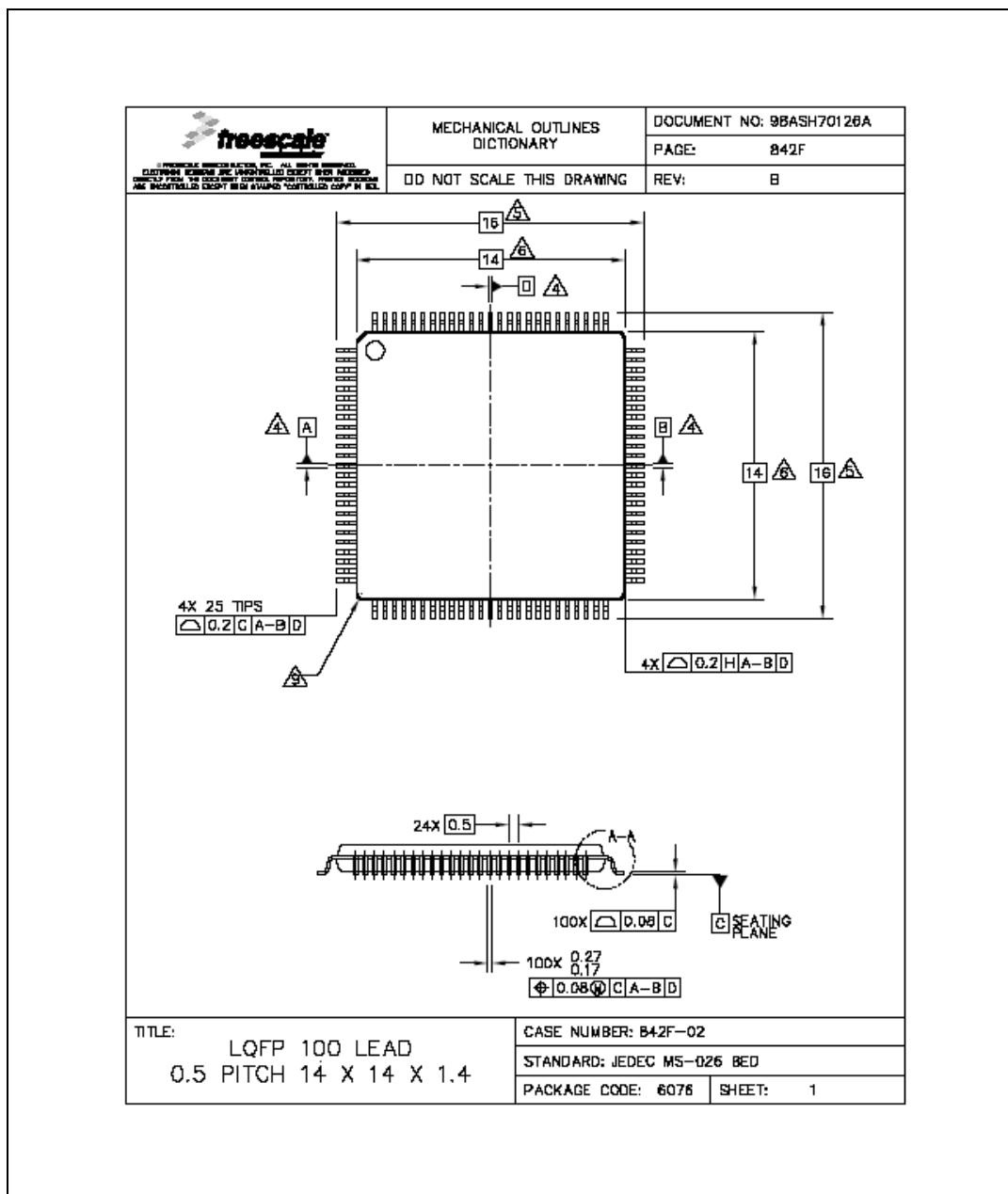
Figure 38. 100 LQFP package mechanical drawing (Part 1 of 3)
