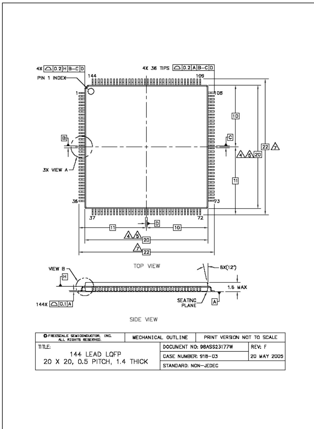
Figure 36. 144 LQFP package mechanical drawing (Part 1 of 2)
