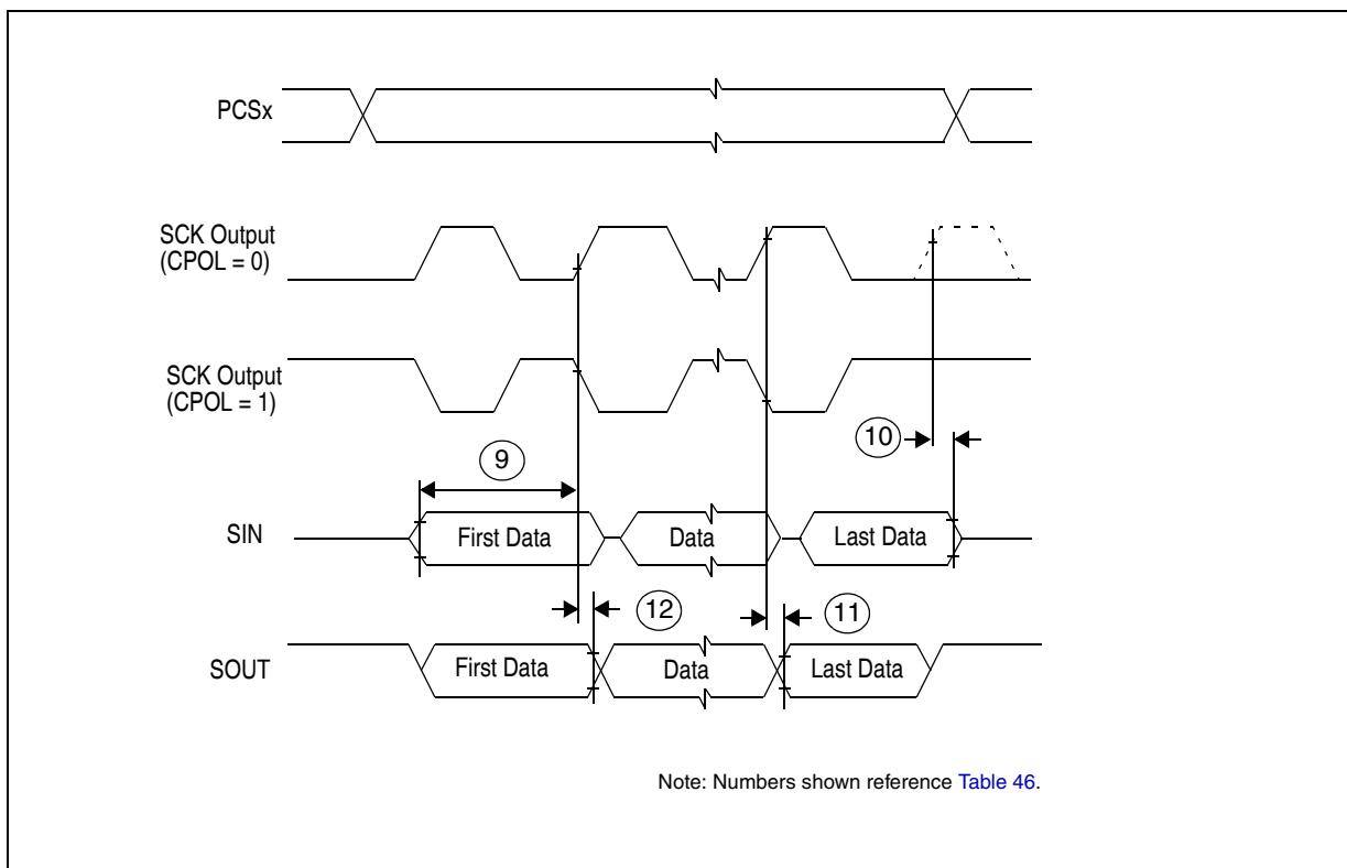
**Figure 27. DSPI modified transfer format timing — master, CPHA = 1**
