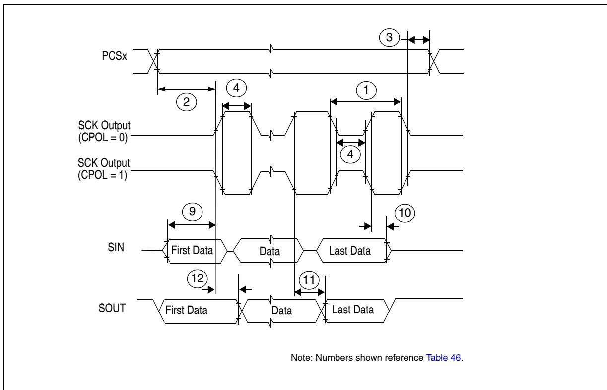
**Figure 26. DSPI modified transfer format timing — master, CPHA = 0**
