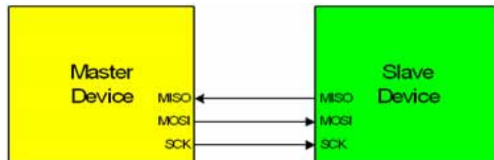
Figure 24.3. 3-Wire Single Master and 3-Wire Single Slave Mode Connection Diagram
