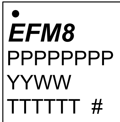
Figure 7.3. QFN32 Package Marking
