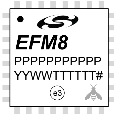
Figure 8.3. QFP32 Package Marking
