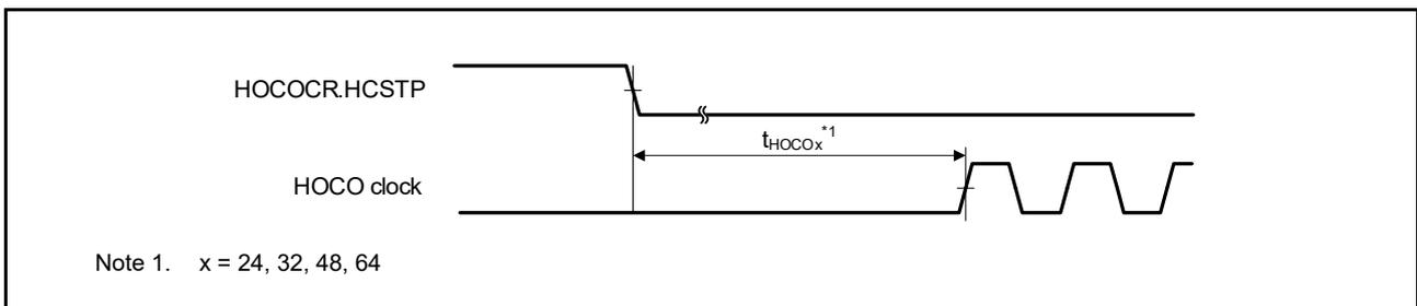
**Figure 2.27** HOCO clock oscillation start timing (started by setting HOCOCR.HCSTP bit)
