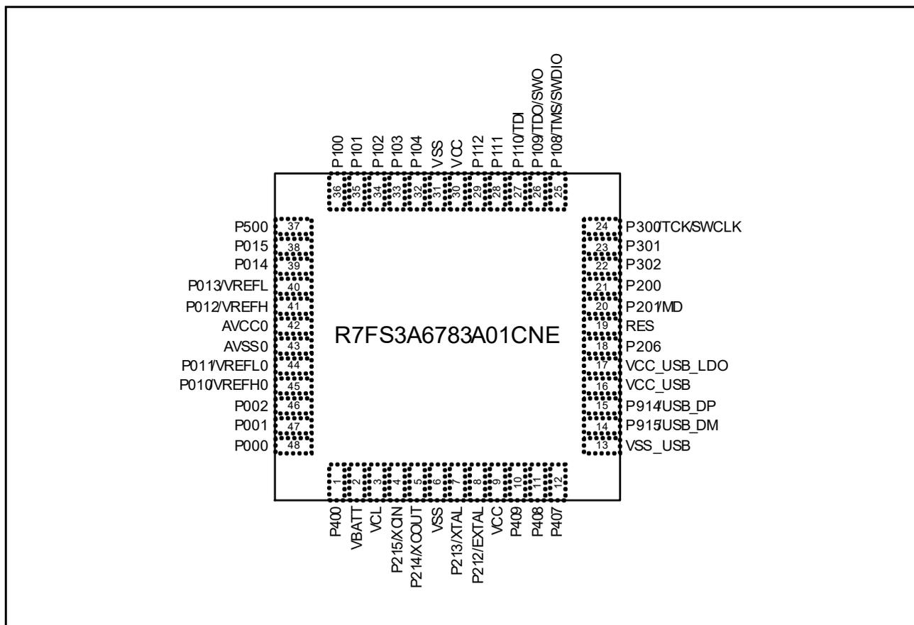
Figure 1.8 Pin assignment for 48-pin QFN (top view)
