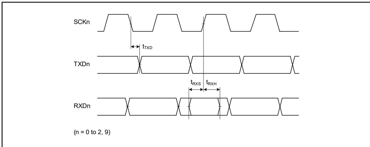
Figure 2.45 SCI input/output timing in clock synchronous mode
