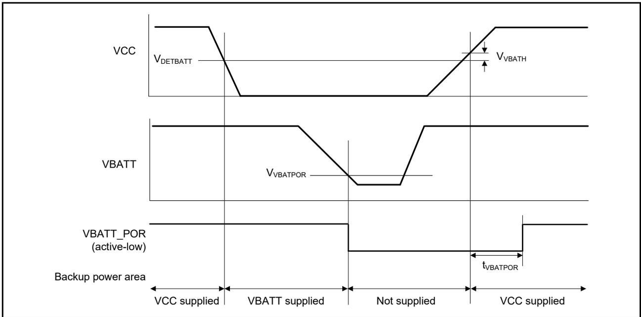
Figure 2.79 VBATT\_POR reset timing
