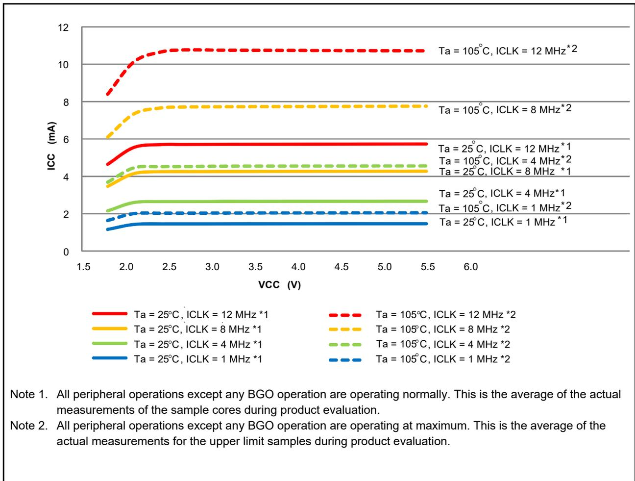
Figure 2.18 Voltage dependency in middle-speed operating mode (reference data)
