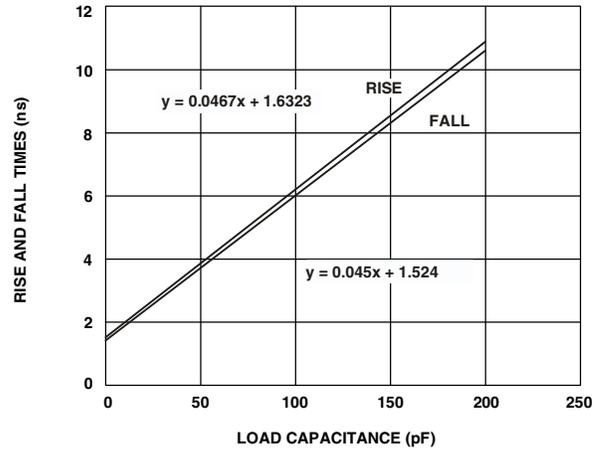
Figure 40. Typical Output Rise/Fall Time (20% to 80%, V<sub>DDEXT</sub> = Max)
