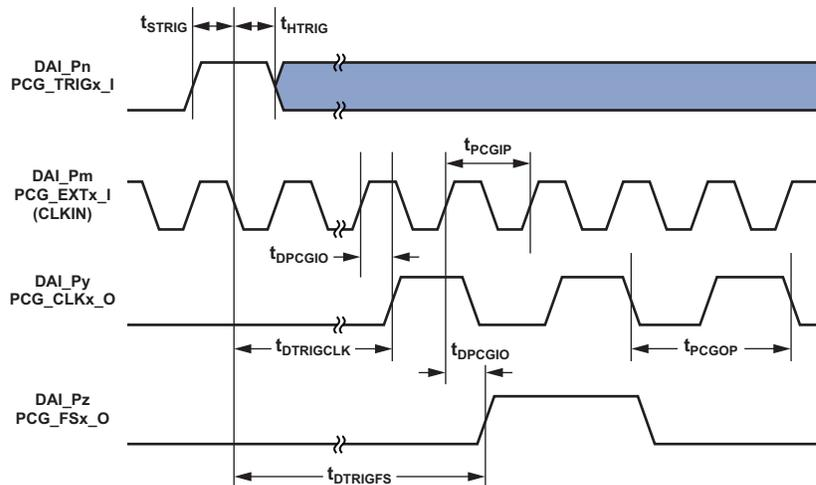
Figure 15. Precision Clock Generator (Direct Pin Routing)
