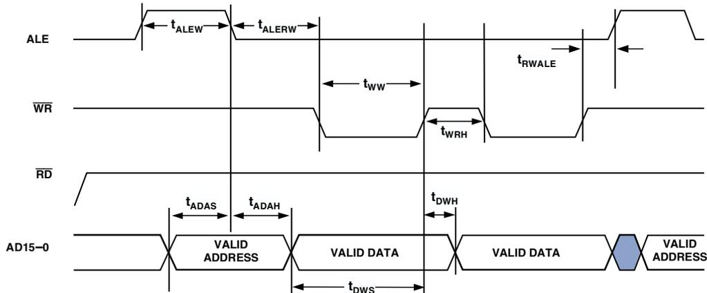
NOTE: FOR 16-BIT MEMORY WRITES, WHEN EMPP  $\neq$  0, ONLY ONE  $\overline{WR}$  PULSE OCCURS BETWEEN ALE CYCLES. WHEN EMPP = 0, MULTIPLE  $\overline{WR}$  PULSES OCCUR BETWEEN ALE CYCLES. FOR COMPLETE INFORMATION, SEE THE ADSP-2136x SHARC PROCESSOR HARDWARE REFERENCE.
