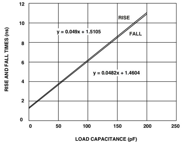
Figure 41. Typical Output Rise/Fall Time (20% to 80%, V<sub>DDEXT</sub> = Min)
