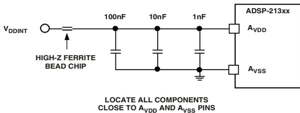
Figure 3. Analog Power ( $A_{VDD}$ ) Filter Circuit
