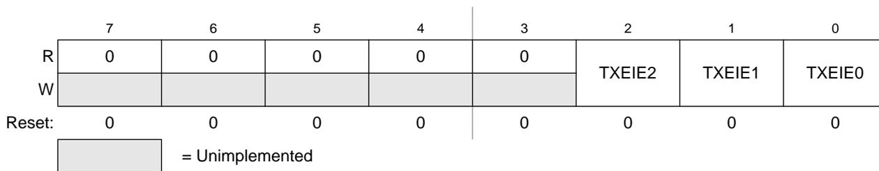
**Figure 12-11. MSCAN Transmitter Interrupt Enable Register (CANTIER)**
