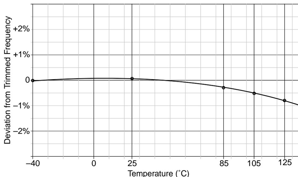
Figure A-9. Typical Frequency Deviation vs Temperature (ICS Trimmed to 16MHz bus @ 25°C, 5V, FEI)<sup>1</sup>
