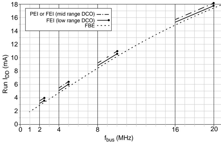
**Figure A-5. Typical Run I<sub>DD</sub> vs. Bus Frequency (V<sub>DD</sub> = 5V)**
