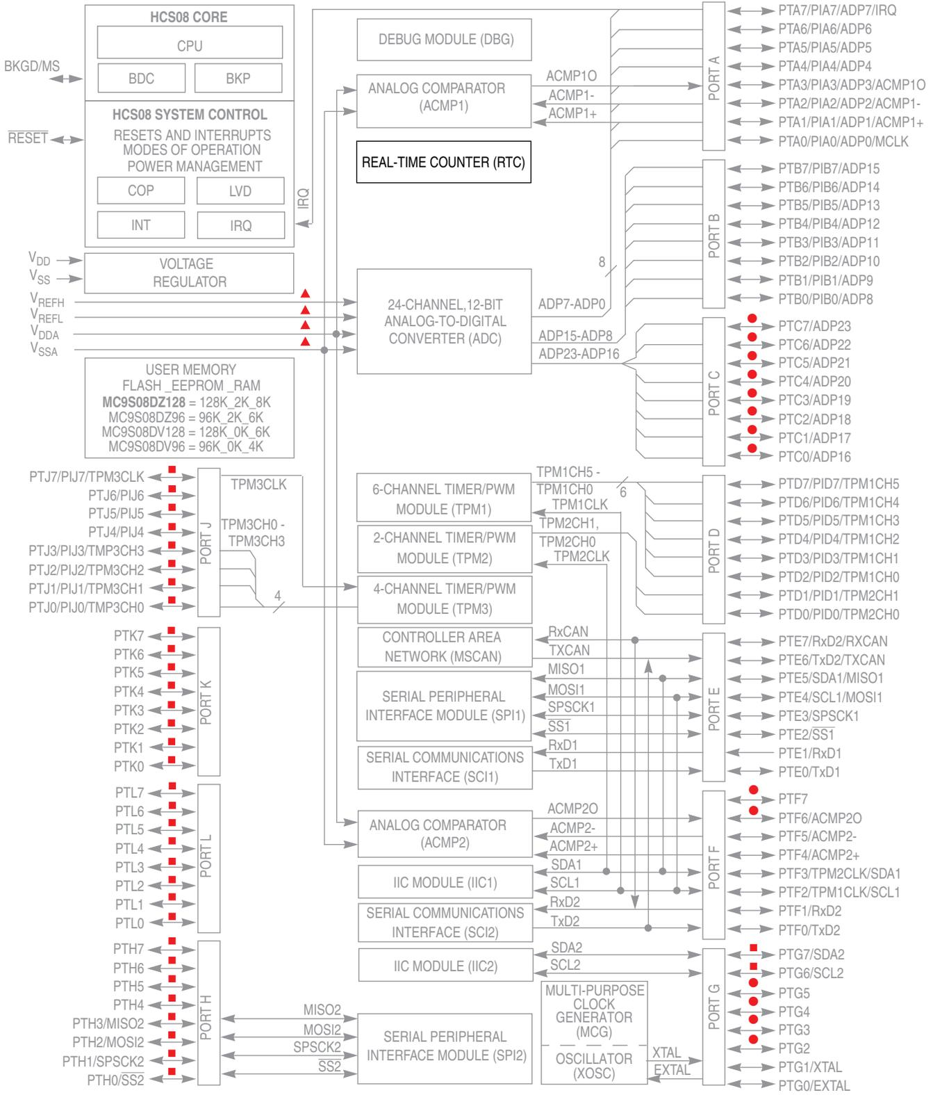
■ - Pin not connected in 64-pin and 48-pin packages    ● - Pin not available in the 48-pin package
