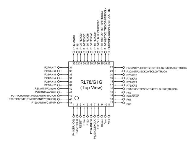
Caution Connect the REGC pin to Vss pin via a capacitor (0.47 to 1  $\mu$ F).
