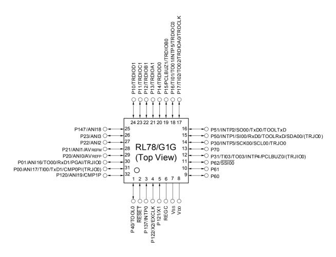
Caution Connect the REGC pin to Vss pin via a capacitor (0.47 to 1  $\mu$ F).
