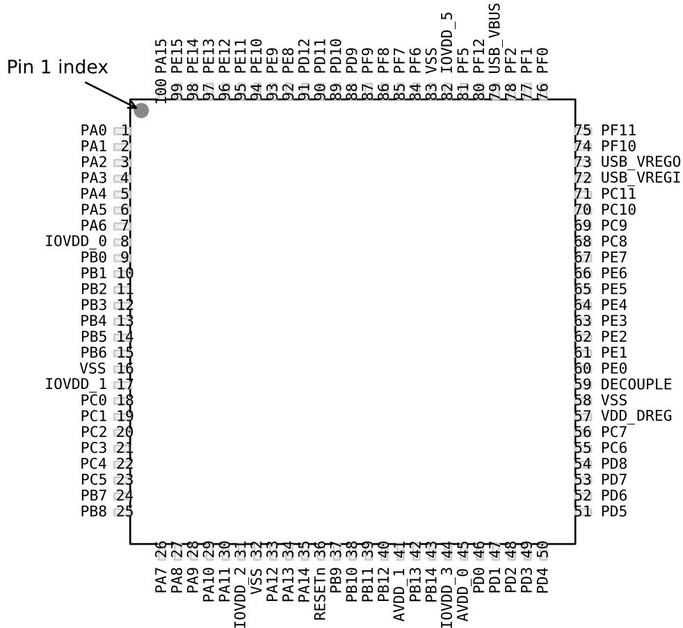
Figure 5.39. EFM32LG980 Pinout (top view, not to scale)
