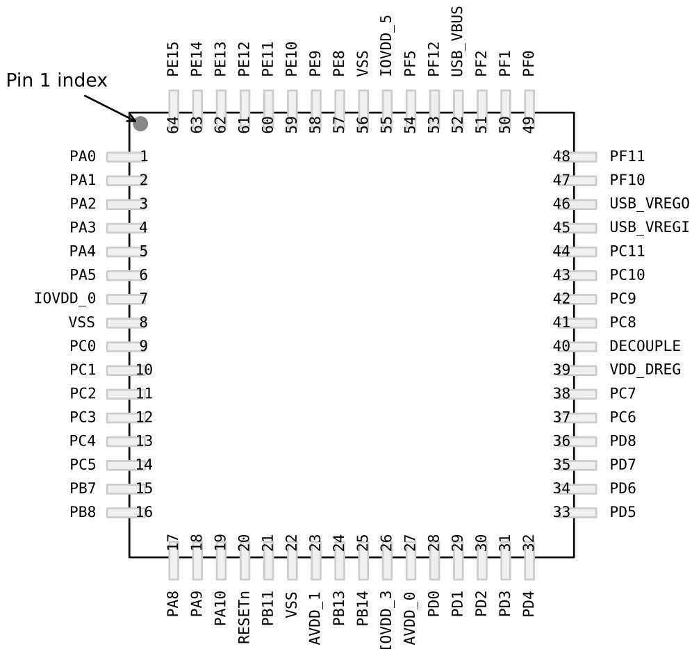
**Figure 5.13. EFM32LG332 Pinout (top view, not to scale)**
