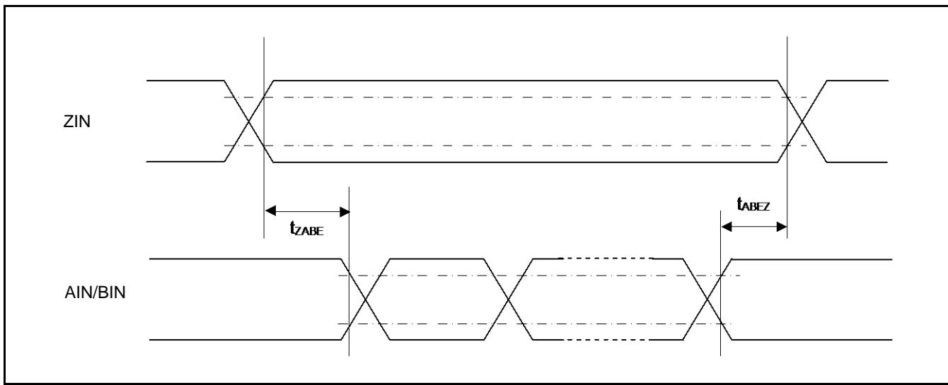
**12.4.20 High-Speed Quad SPI Timing**
