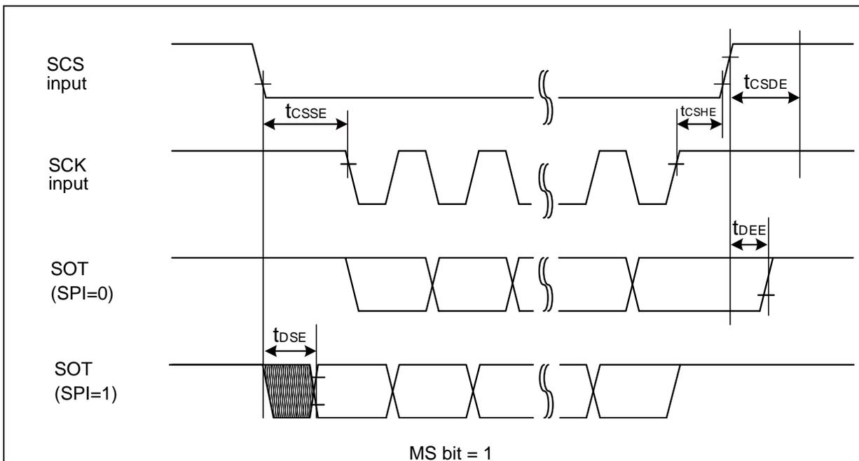
**High-Speed Synchronous Serial (SPI = 1, SCINV = 1)**
