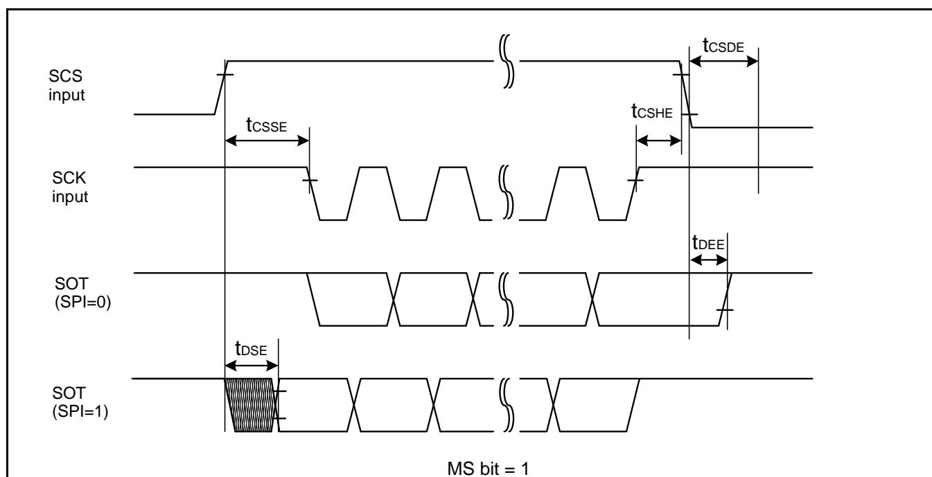
**High-Speed Synchronous Serial (SPI = 0, SCINV = 1)**
