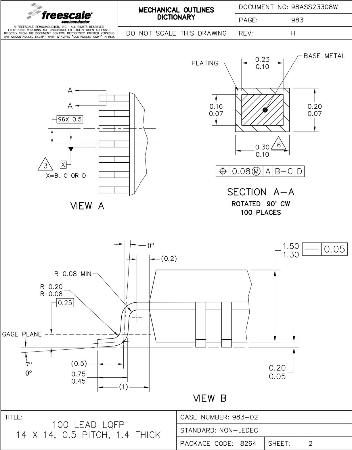
Figure 39. 100 LQFP package mechanical drawing (2 of 3)
