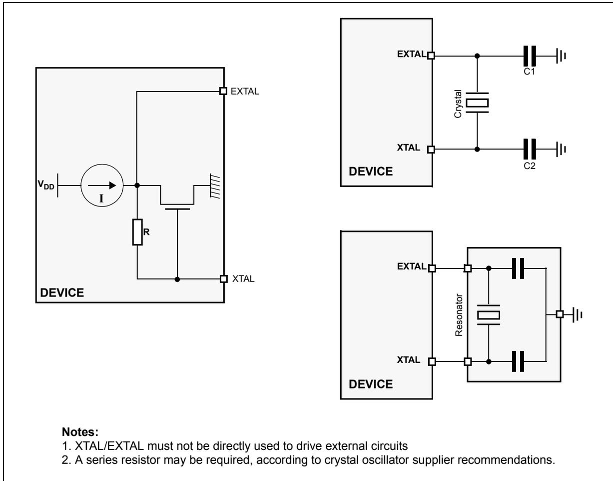
Figure 14. Crystal oscillator and resonator connection scheme
