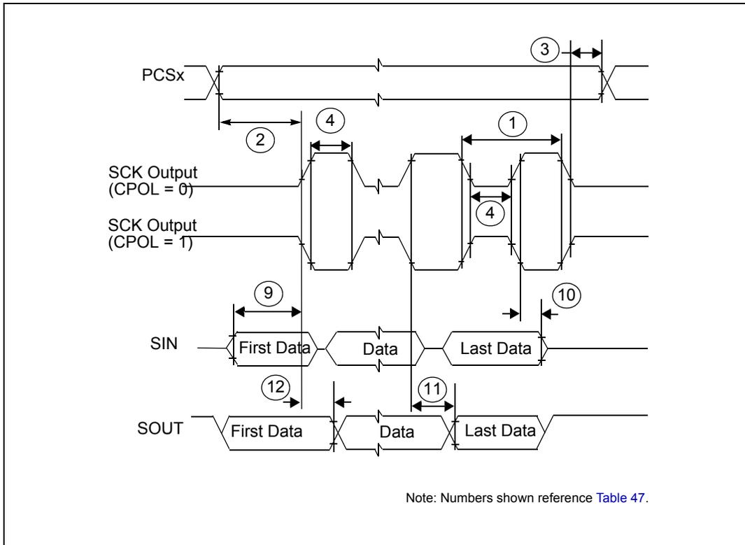
Figure 28. DSPI modified transfer format timing – master, CPHA = 0
