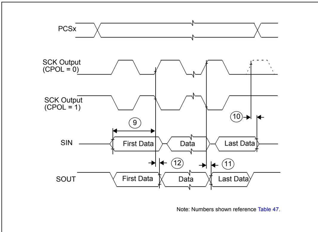
Figure 29. DSPI modified transfer format timing – master, CPHA = 1
