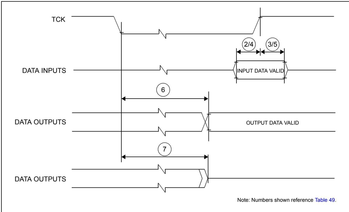
Figure 34. Timing diagram – JTAG boundary scan
