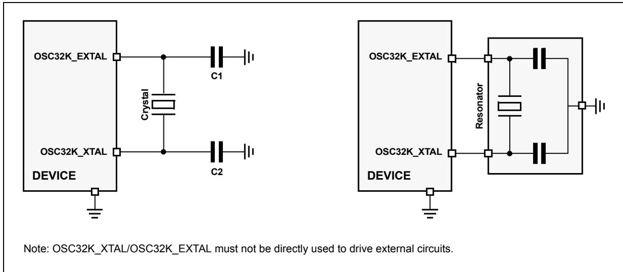
Figure 16. Crystal oscillator and resonator connection scheme
