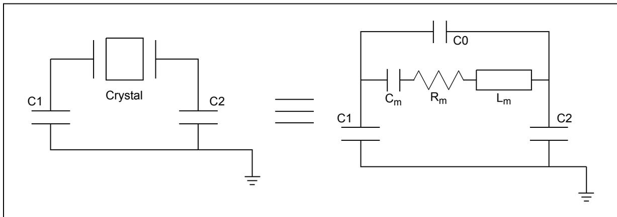
Figure 17. Equivalent circuit of a quartz crystal
