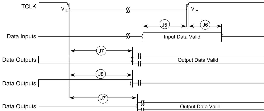
Figure 24. Boundary Scan (JTAG) Timing
