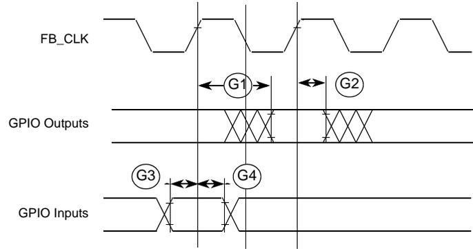
Figure 13. GPIO Timing
