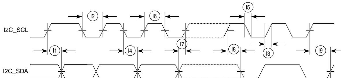
**Figure 17. I<sup>2</sup>C Input/Output Timings**
