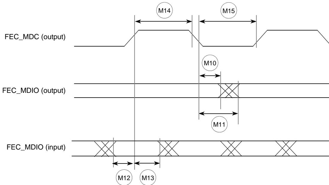
Figure 21. MII Serial Management Channel Timing Diagram
