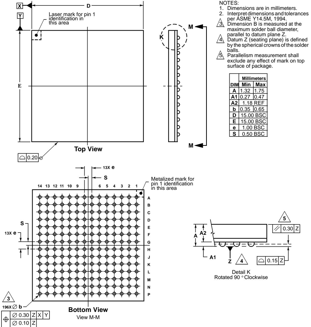
Figure 31. 196 MAPBGA Package Dimensions (Case No. 1128A-01)
