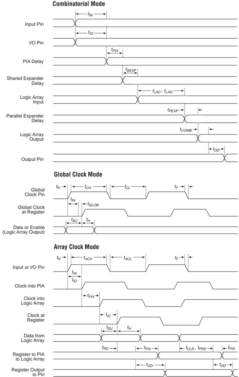
**Table 18. EPM7032AE Internal Timing Parameters (Part 2 of 2)** *Note (1)*
