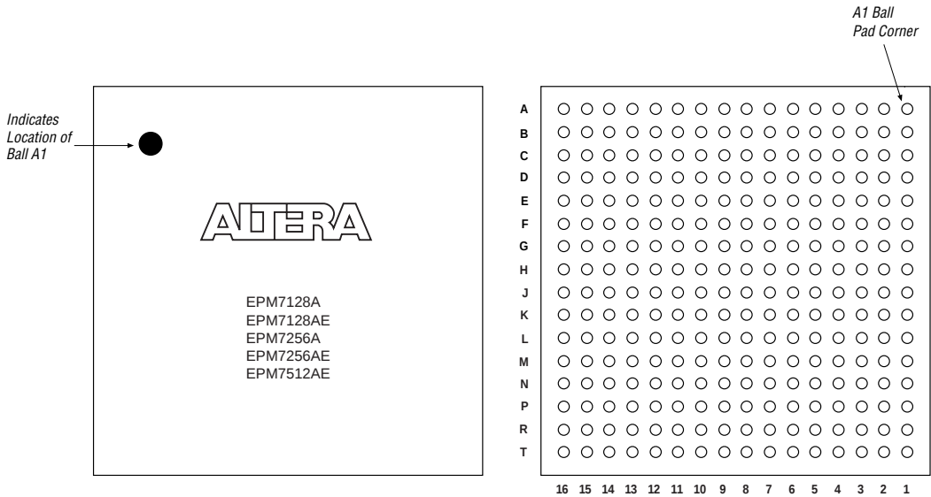
Figure 23. 256-Pin FineLine BGA Package Pin-Out Diagram
