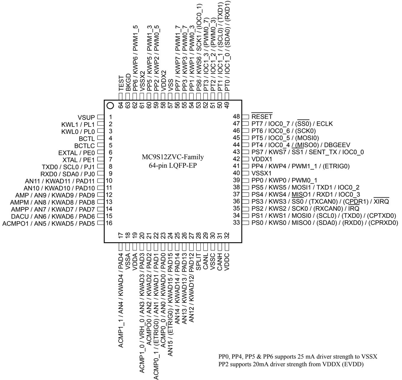
1. The exposed pad on the package bottom must be connected to a ground pad on the PCB.
