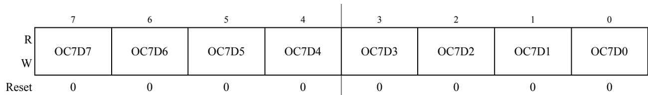
Figure 11-9. Output Compare 7 Data Register (OC7D)
