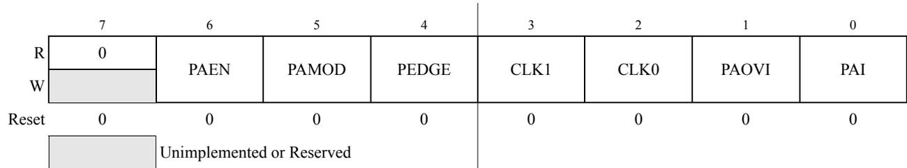
**Figure 11-24. 16-Bit Pulse Accumulator Control Register (PACTL)**
