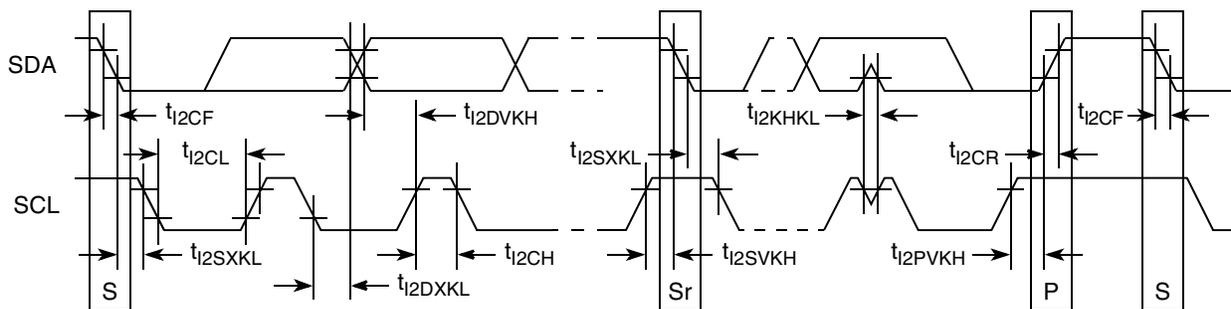
**Figure 31. I<sup>2</sup>C bus AC timing diagram**
