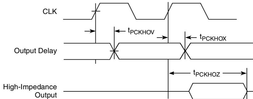
Figure 25. PCI output AC timing measurement condition
