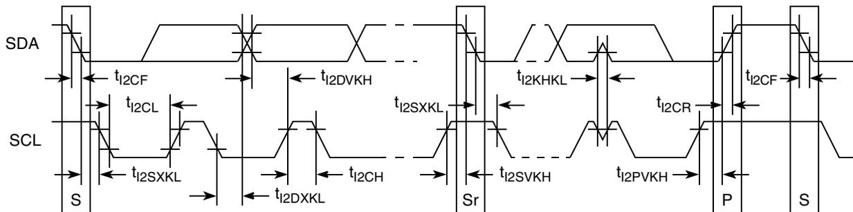
**Figure 31. I<sup>2</sup>C bus AC timing diagram**
