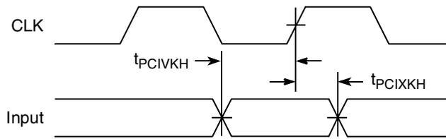
Figure 24. PCI input AC timing measurement conditions
