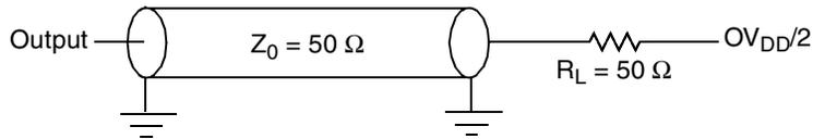
Figure 7. Enhanced local bus ac test load
