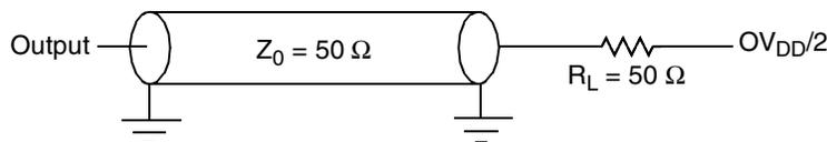
**Figure 32. Timers AC test load**
