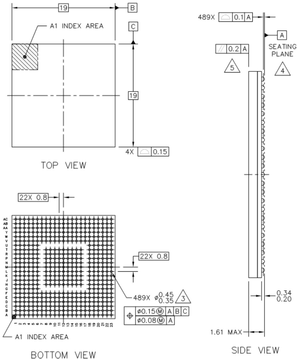
Figure 42. Mechanical dimensions and bottom surface nomenclature of the MPC8309 MAPBGA
