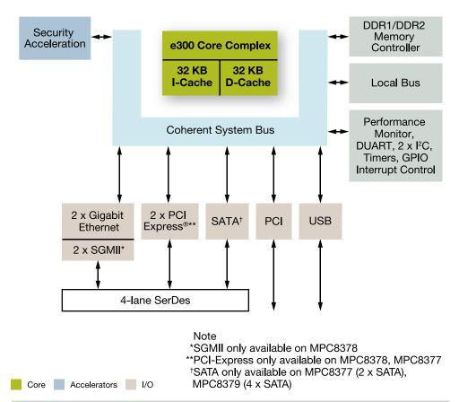
and supports either x1 or x2 widths, making it an excellent choice for wireless access points and low-end printers. The integrated SATA controllers support both SATA I and II data rates (1.5 and 3.0 Gbaud), providing integrated support for hard disk drive applications such as network attached storage.
