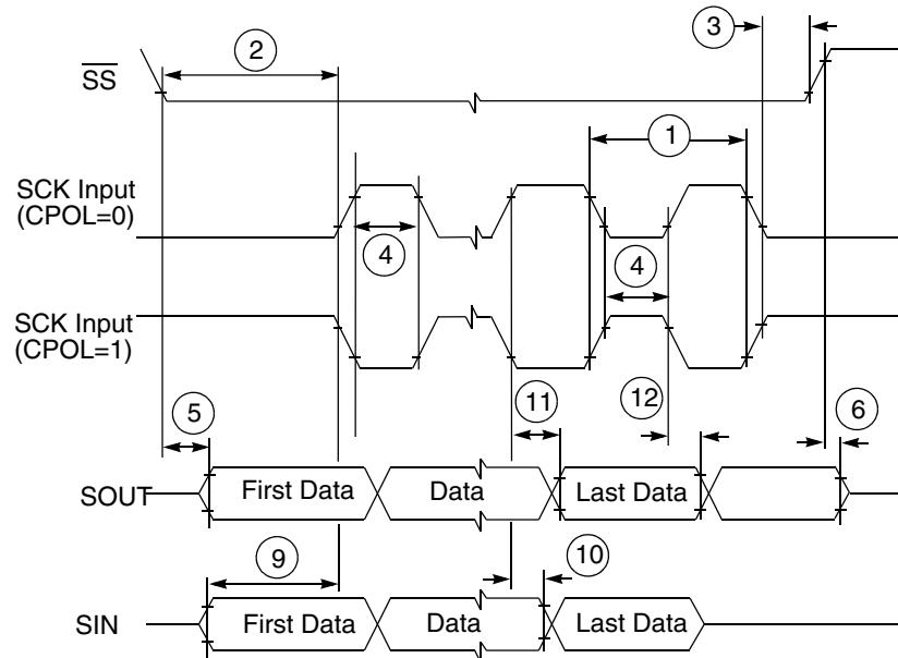
**Figure 27. DSPI modified transfer format timing – slave, CPHA = 0**
