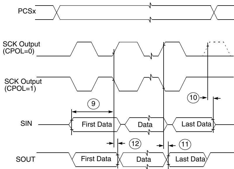
**Figure 26. DSPI modified transfer format timing — master, CPHA = 1**
