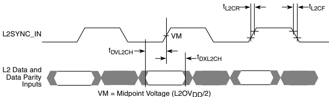
Figure 8. L2 Bus Input Timing Diagrams
