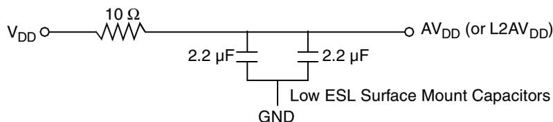
**Figure 21. PLL Power Supply Filter Circuit No.1**
