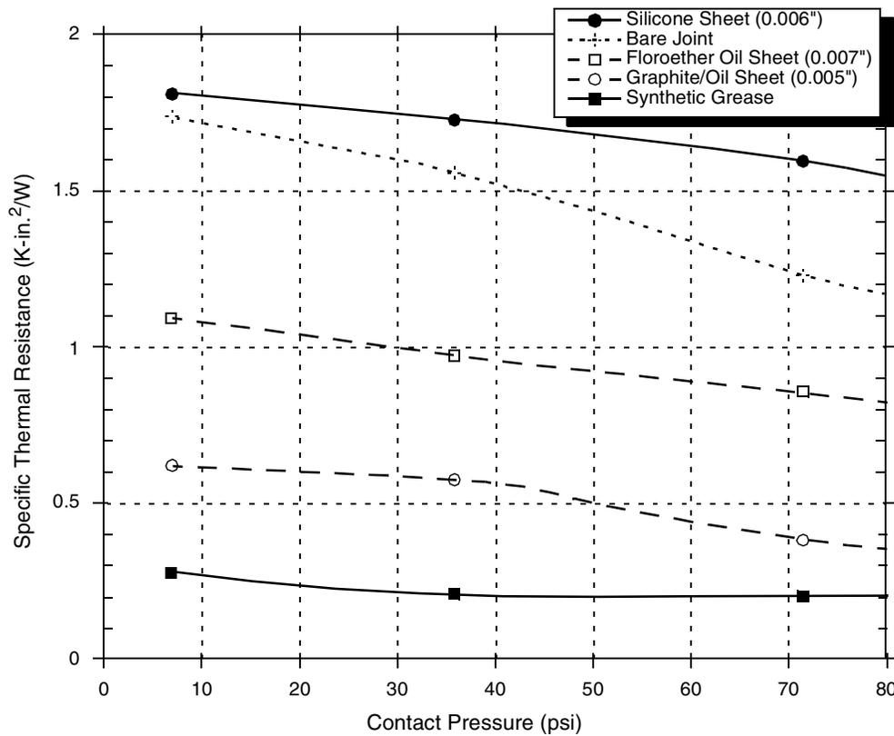
**Figure 29. Thermal Performance of Select Thermal Interface Material**
