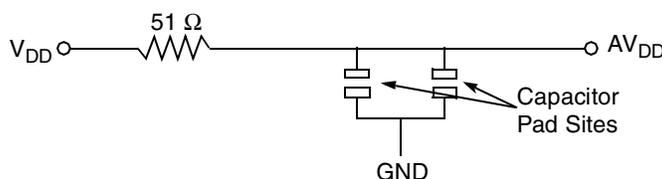
**Figure 22. PLL Power Supply Filter Circuit No. 2**
