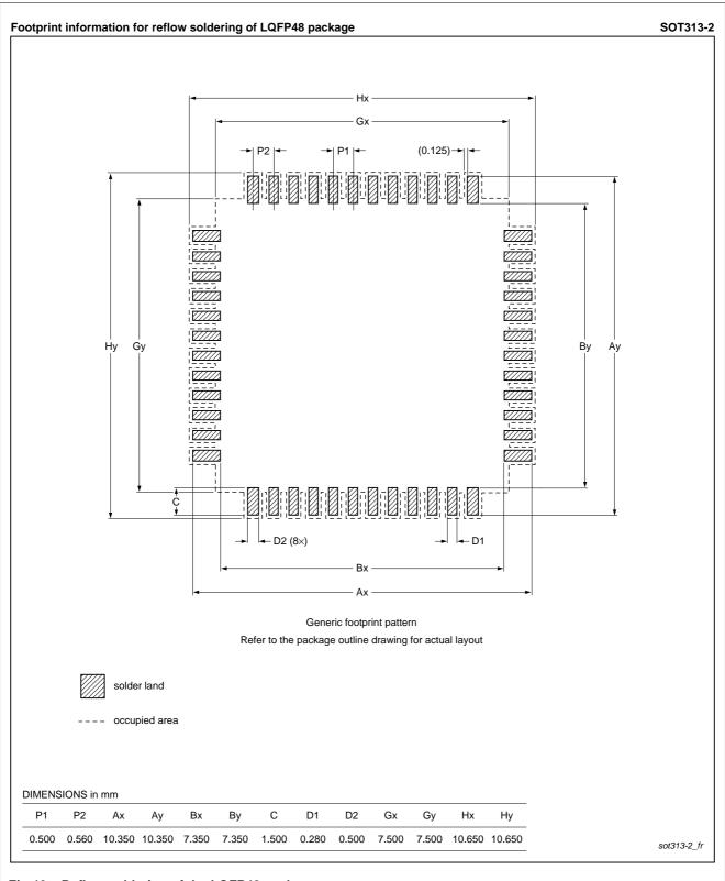
Fig 40. Reflow soldering of the LQFP48 package
