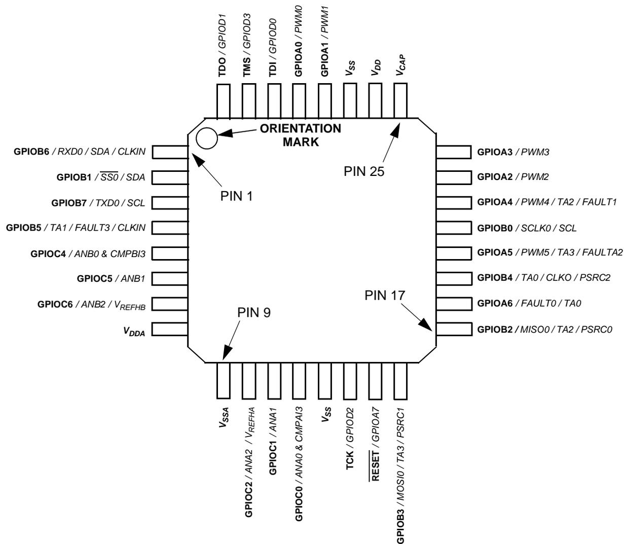
Figure 11-1 Top View, 56F8033/56F8023 32-Pin LQFP Package
