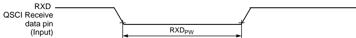
Figure 10-12 RXD Pulse Width
