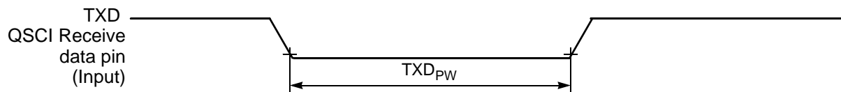
Figure 10-13 TXD Pulse Width
